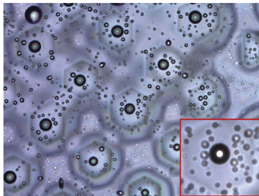
Figure 4. Microscope image of sample B after about 1 hour of cooling, in the LC lens' focal plane (from reference [37]).
